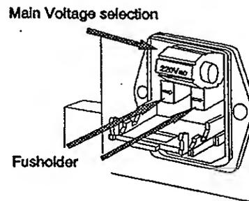
Use a screw driver to open the power plug enclosure. Pull out the fuse holders to exchange the fuses.
